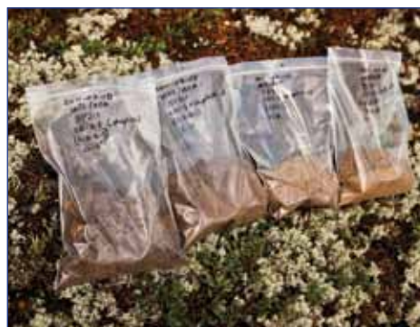
Soil samples from each plane of a soil pit.
