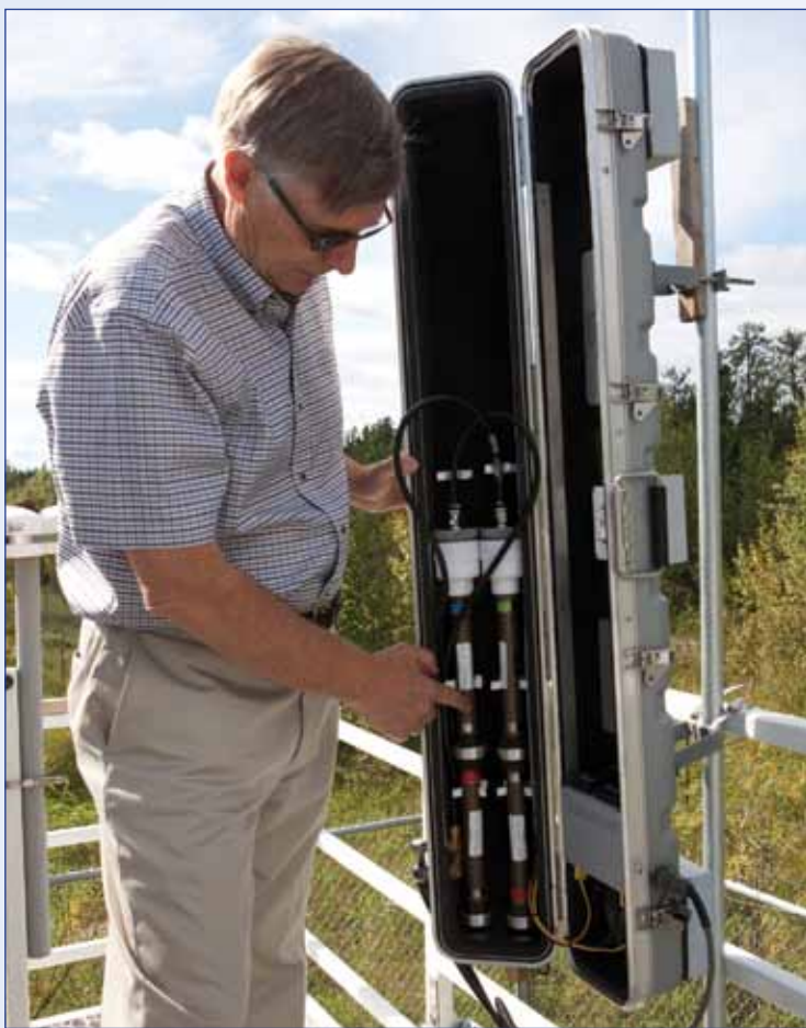
Left: Dr Kevin Percy inspects an Annular Denuder, which measures acidic and basic gases at AMS #1 Fort McKay.
