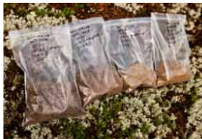
Soil samples from each plane of a soil pit.
